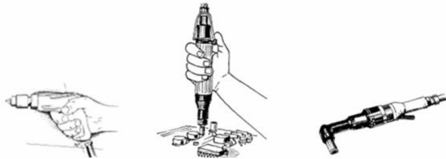
Figure 6.36: Power tool examples - Pistol Grip (Left), In-Line (Center), and Right Angle (Right)
