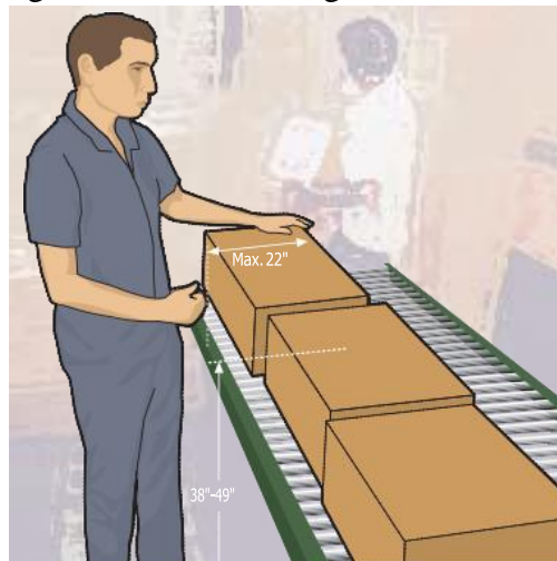
Figure 6.15: Work height and reach distances
